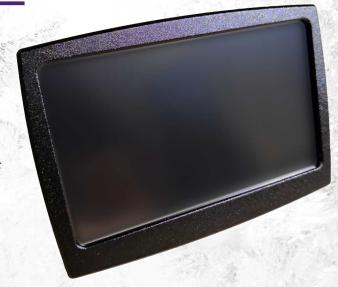
Thanks to it's microcontroller-based electronics, **UVOD** is lightning fast to boot up. When traditional industrial displays take multiple seconds, or dozens of seconds to boot up, **UVOD** can initialize itself in less than a second.
